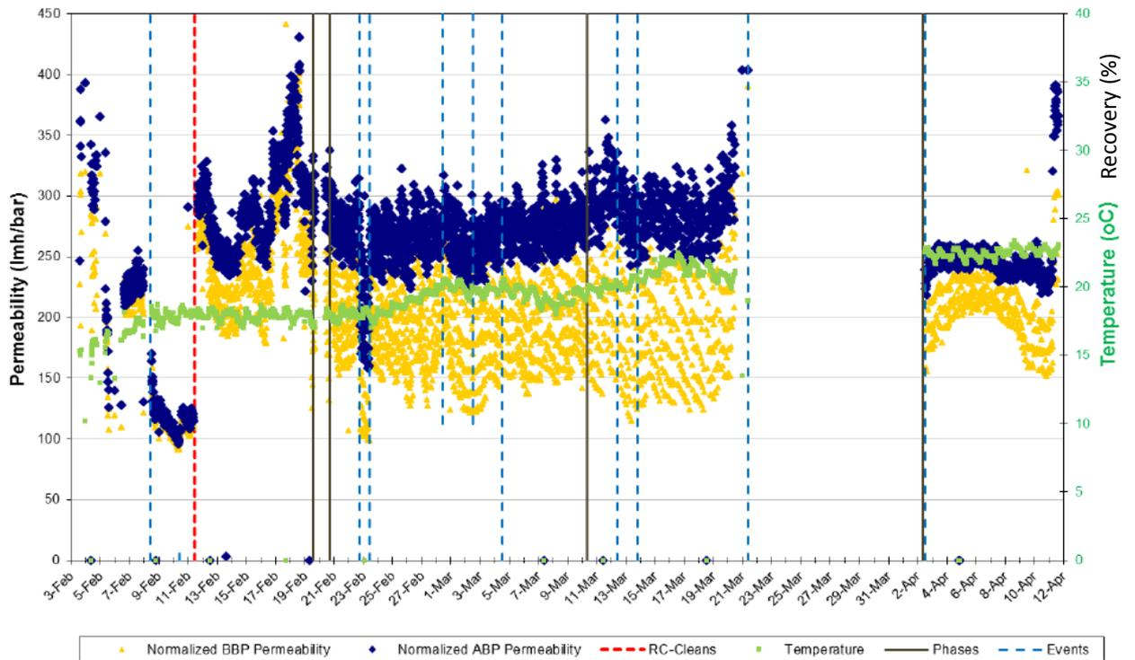
Figure 3: Temperature Corrected Permeability profile for the entire pilot study
