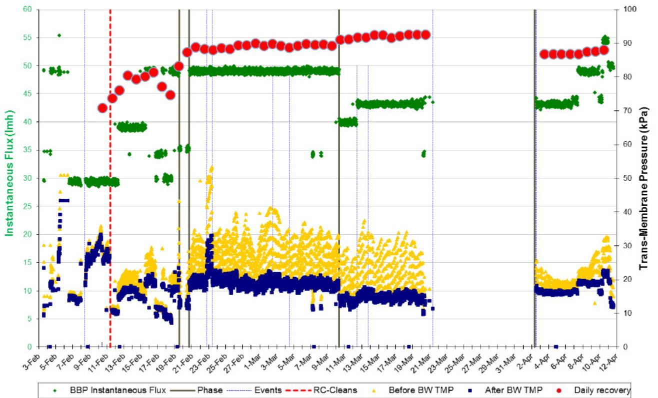
Figure 2 : UF Flux, TMP and recovery for the entire pilot study
